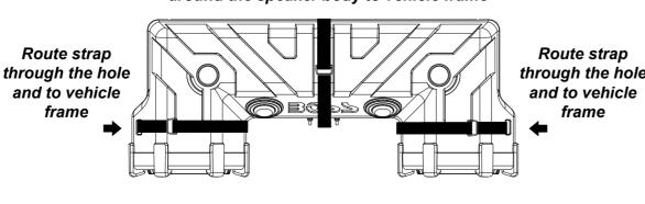
**CAUTION!!** Mounting straps should be double checked to be sure they are pulled tight and secure before each use of the vehicle.
